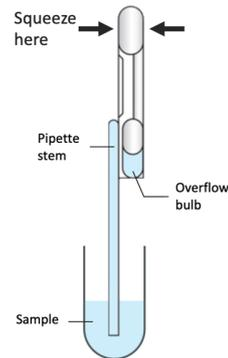
**Figure 2.** Transfer Pipette
